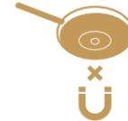
To determine whether a pot is suitable, a magnet may be used to check whether pots are magnetic.
