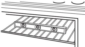
3. If range is not level, adjust the leveling rods. Using a wrench, turn leveling rods located behind the kick plate to level range and to raise or lower range to the desired countertop height. Leveling rods can be adjusted up to 1½" (3.9 cm).
