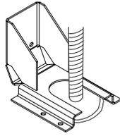
2. Move range into its final location, making sure rear leveling leg slides into anti-tip bracket.
